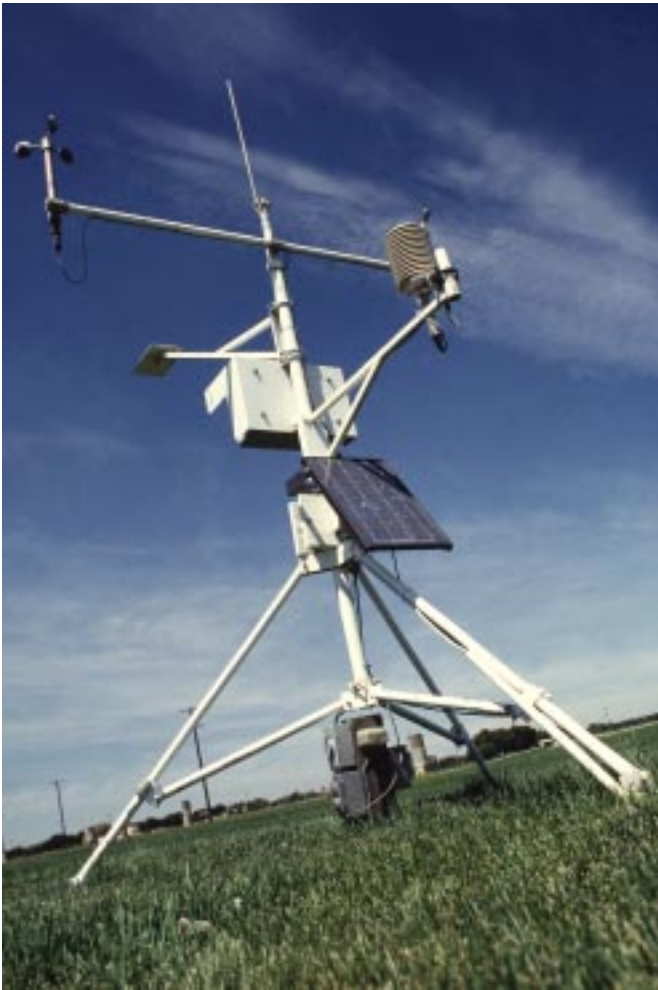
A specialized weather station (CIMIS station) or a Class A evaporation pan (background) can be used to determine reference evapotranspiration (ET o ) for a site. Daily CIMIS data is available online at www.cimis.water.ca.gov .
